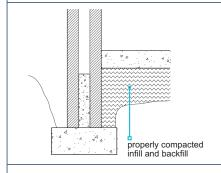
The total compacted hardcore thickness should generally be in the range of 100-600mm. (NHBC Standards Clause 5.1.8)
