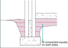
Fill should be placed in layers of equal thickness to both sides of substructure walls so that compaction on one side is not more than one layer ahead of the other.
